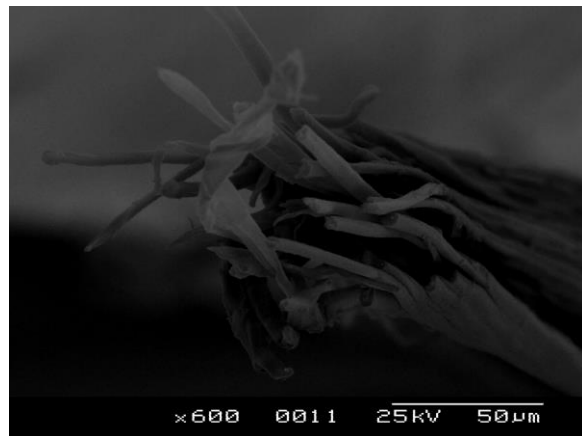
Figure 5: cross-section of Typha stem fiber at the optimum conditions
