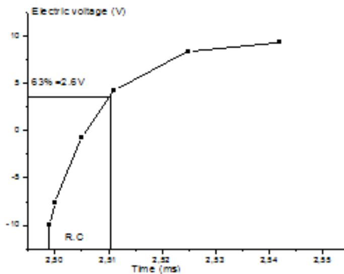
Figure 3: Determination of the time constant  $\zeta = RC$  for the sample N°1.
