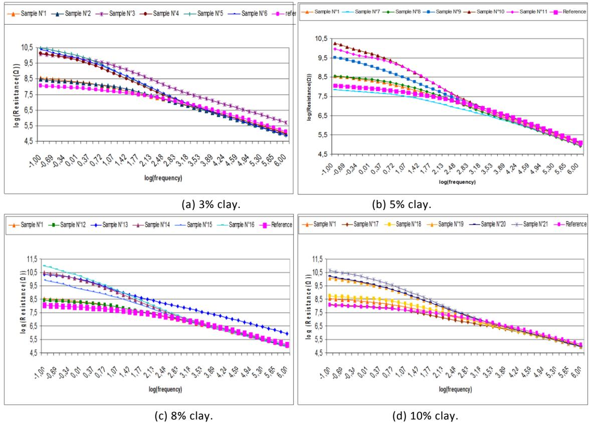
Figure 6 (a-d): Electric resistance at different clay percentages and different dropped quantities.
