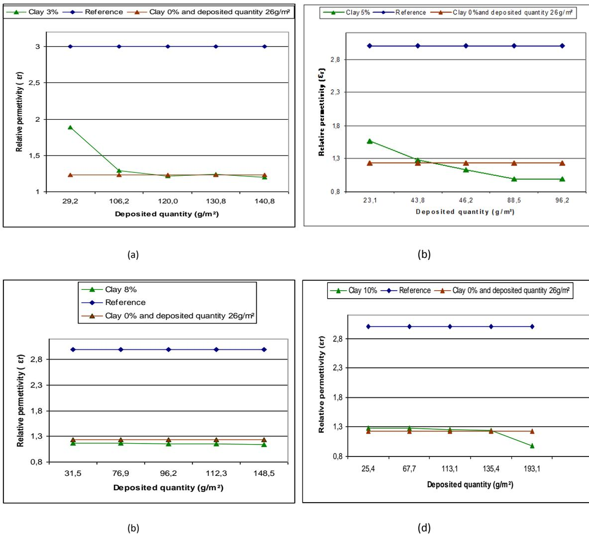
Figure 4 (a-d): Relative permittivity at different clay percentages and different deposited quantities.
