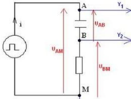
Figure 2: Measurement of the capacitance.
