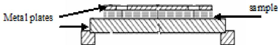
Figure 1: Condenser: two metal plates and the fabric inside.
