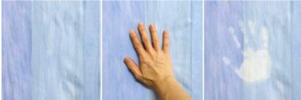
Figure 7: Thermo-reactive property of the coating
