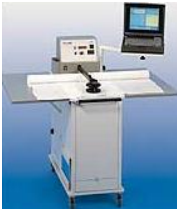
Figure 4 : Air Permeability Tester TEXTEST FX 3300
