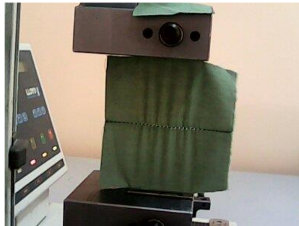
Figure 2: Seam slippage test
