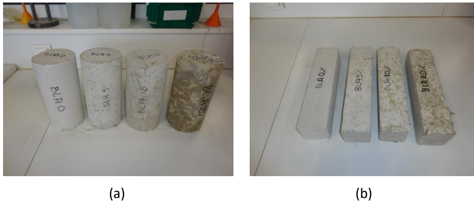
Figure 5: (a) ALC specimens for compressive tests. (b) ALC specimens for thermal tests.
