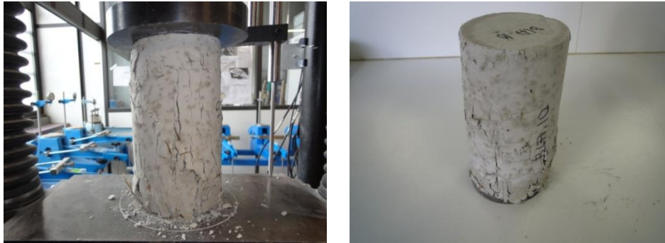
Figure 6: Example of ALC10% specimen during and after compression test.
