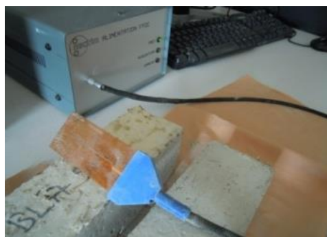
Figure 7: Hot-wire transient method.
