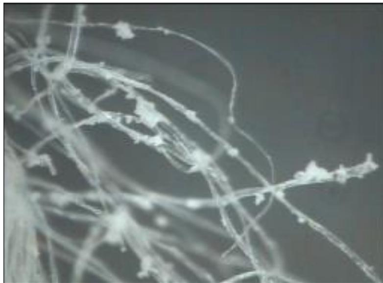
Figure 8: SEM micrographs of impregnated textile substrates
